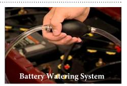
The battery watering system makes maintaining the batteries so much easier!
